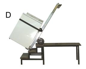
Repeat the above steps 2 and 3, until the bottom of the stairs are reached. Note: The *PowerMate*<sup>®</sup> can be "parked" on the stairs in a balance position spanning two steps, at any interval as shown in "D".
